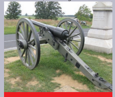
10-pounder Parrott rifle (note reinforced banding at the breech)
